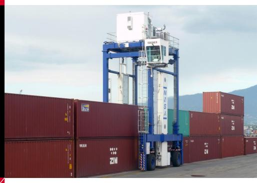
Isoloader's Transporter Straddle Carrier is used by L-3 Corporation in their RDSC solution for scanning containers for nuclear weapons. It meets the US Dept. of Energy's requirements for operating in extreme conditions. Isoloader's straddle carriers and rubber tyred gantries are designed to handle extreme environmental, including dust, heat and cold.
